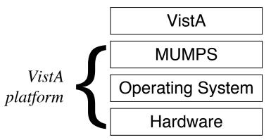
Figure 1: VistA source code and supporting platform
